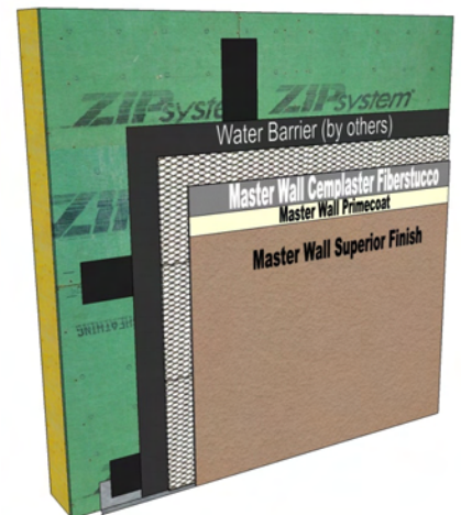
Cemplaster Fiberstucco over slip sheet. Drainage Mat is optional
