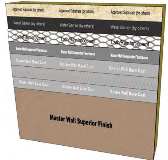
Bulltec Stucco Mesh Embedded in Master Wall® Base Coat
