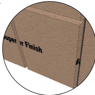
3/4" deep by 3/4" wide (19 x 19 mm) V-groove shown
