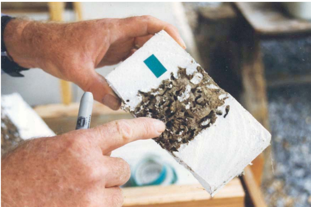
#45 TEST FIXTURE - Close-up shows termite nesting galleries formed in non-treated EPS.
