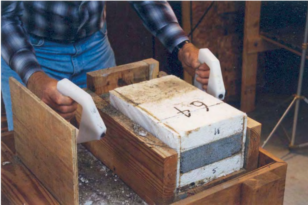
#64 TEST FIXTURE - Examination of Perform Guard EPS after 3 years exposure. Highland site, Mississippi.
