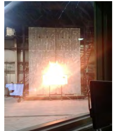
Ultra-Lath Plus® undergoing NFPA 285 testing
