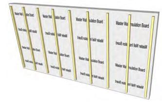
Apply ribbons vertically about 6" (152 mm) apart with 3/8" (9.5 mm) tall adhesive beads. Keep adhesive about 3/4" (19 mm) away from edges and gently place board in place.
