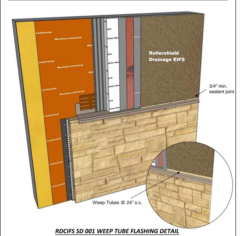
These drawings relay the conceptual conditions of Master Wall<sup>®</sup> Systems and are not the construction drawings. Ultimately the design and detailing of an entire wall system is the responsibility of a professional. These details will guide the design professional in the use of Master Wall<sup>®</sup> Products. Master Wall disclaims design, warranty or construction intent or responsibility. **Bold = Master Wall<sup>®</sup> Product.** ©2014 Master Wall Inc.<sup>®</sup>
