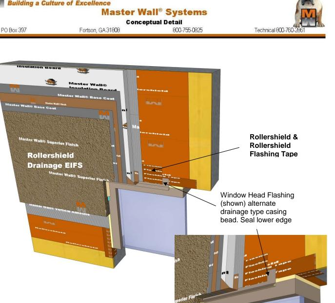
1/2" (12.7 mm) min. fillet-type sealant joint Flush Window installed and sealed per window manufacturer's requirements
