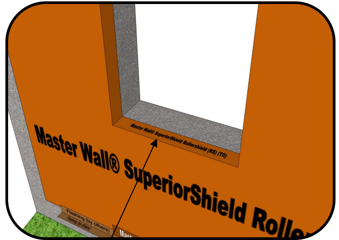
Turn Rollershield into opening at least as far as the end of the window unit so it may be sealed (by others)
