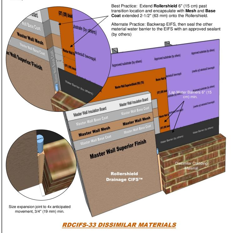
Model Link: <u>https://3dwarehouse.sketchup.com/model/933be7e4-65a7-4101-a3e7-f7573b169835/Rollershield-</u> Drainage-CIFS%E2%84%A2-Detail-at-Dissimilar-Materials
